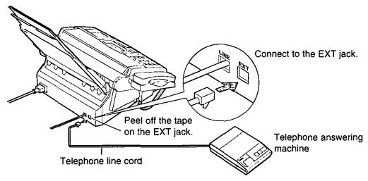
Set the number of rings on the telephone answering machine to less than 4.
